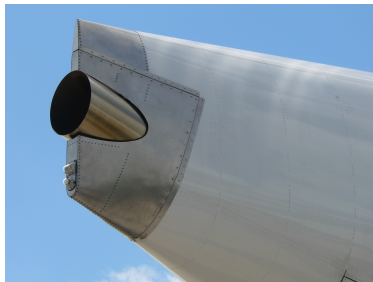
APU on an Airbus A380
