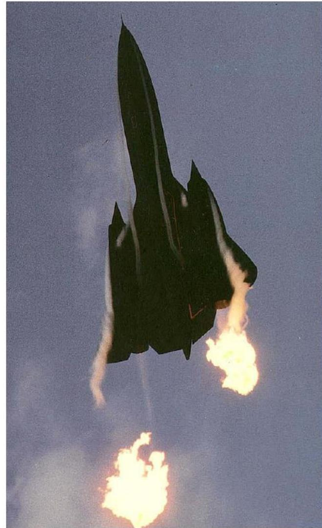
Flame blowoff in the SR-71 during a high-acceleration turn, Campbell and Chambers
