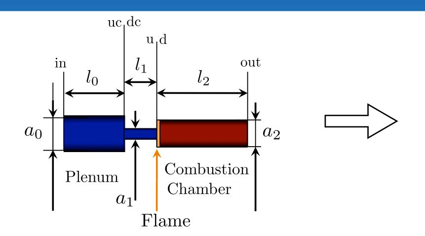
$$\begin{bmatrix} f_{\text{out}} \\ g_{\text{out}} \end{bmatrix} = \underbrace{\begin{bmatrix} T_{11}(s) & T_{12}(s) \\ T_{21}(s) & T_{22}(s) \end{bmatrix}}_{T(s)} \begin{bmatrix} f_{\text{in}} \\ g_{\text{in}} \end{bmatrix}.$$
