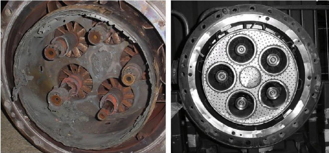
Burner assembly damaged by combustion instabilities (left). New assembly (right). Goy et al. 2005
