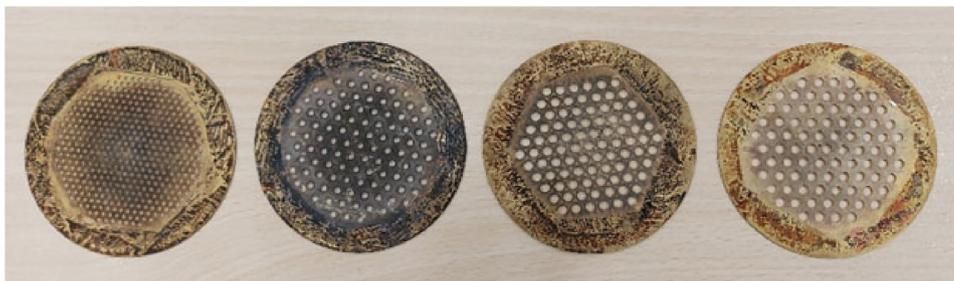
**Figure 7.** Burners under study (Burners B<sub>15</sub>, B<sub>2</sub>, B<sub>3a</sub> and B<sub>3b</sub> from left to right).
