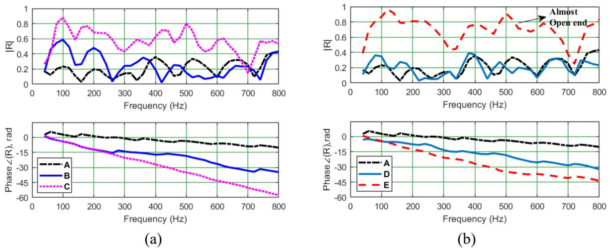
Figure 5: (a) Reflection Coefficient for A (Movable piston position: 0 cm, TTL: 0 cm), B (Movable piston position: 0.5 cm, TTL: 18 cm) and C (Movable piston position: 3 cm, TTL: 32 cm) and (b) Reflection Coefficient for A (Movable piston position: 0 cm, TTL: 0 cm), D (Movable piston position: 0 cm, TTL: 53 cm) and E (Movable piston position: 7.2 cm, TTL: 53 cm)
