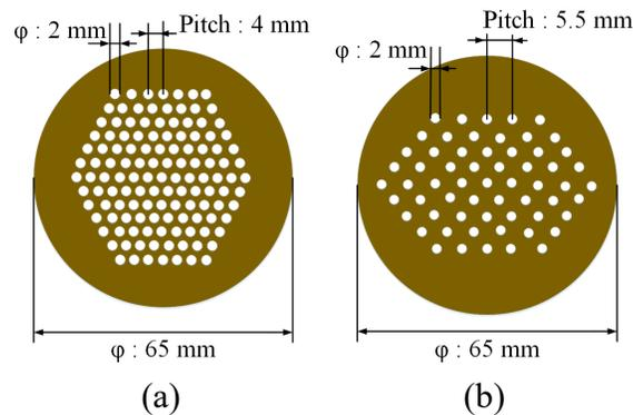
Figure 4: (a) Burner P<sub>4</sub> with Pitch 4 mm and area 398.9 mm<sup>2</sup>, and (b) Burner P<sub>5.5</sub> with Pitch 5.5 mm and area 191.6 mm<sup>2</sup>
