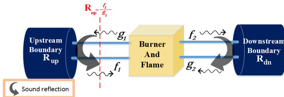
Figure 1: Forward and backward propagating waves in a duct with flame
