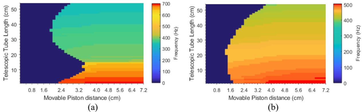
Figure 6: (a) Stability Plot for Burner  $P_4$  and (b) Burner  $P_{5.5}$  colours indicate frequencies (blue i.e. 0 Hz frequency represents stable regime)
