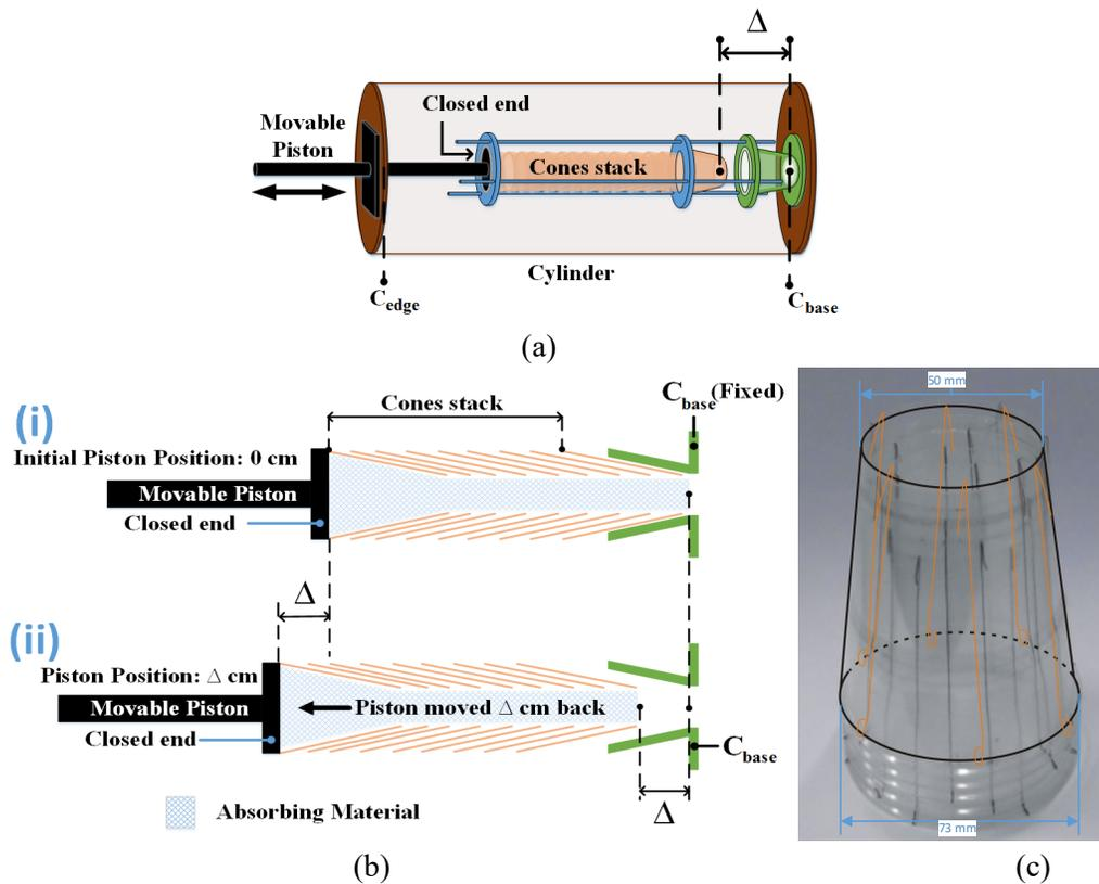
Figure 3: (a) Cylinder with cones stack diagram, (b) 2D representation of initial position of Movable Piston and at  $\Delta$  cm displacement, and (c) truncated hollow cones stack with spacers (4 cones)
