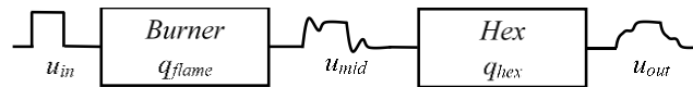
Figure 5.3: A schematic of the network model for the total system showing the excitation and response signals.
