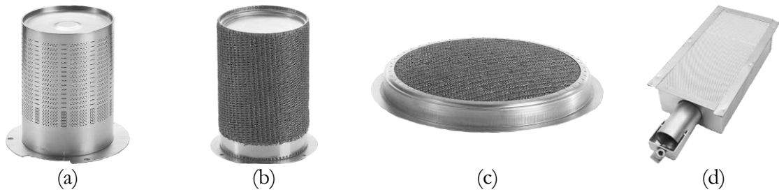
Figure 4.1: Some possible configurations of practical burners, i.e., perforated cylindrical (a), metal fiber cylindrical (b), metal fiber flat (c), and ceramic flat (d) burners (images a, b and c courtesy of Bekaert Combustion Technology B.V., and image d courtesy of American Range Corporate).
