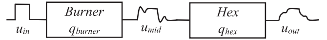
Fig. 3. A schematic of the network model for the total system showing the excitation and response signals.
