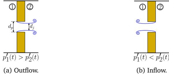
Figure 4.1: Formation of the acoustic jet in orifices. The jet continuously changes direction depending on the pressure difference between the two sides of the orifice where  $d_p$  and  $d_j$  are the orifice and jet cross-section diameters, respectively.
