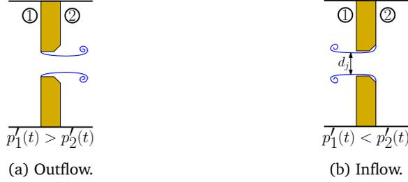
Figure 4.3: The difference of the jet area between the inflow and outflow of an orifice with an asymmetrical edge-profile. For the outflow, the separation occurs at the sharp upstream edge and  $C_v \simeq 0.7$ . For the inflow, the separation takes place downstream and due to the chamfer, the vena contracta factor is  $C_v \simeq 0.95$ .
