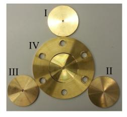
Figure 2.6: Samples used in the impedance tube to verify the numerical model. Samples I, II and III require a sample holder while Sample IV has it built-in.
