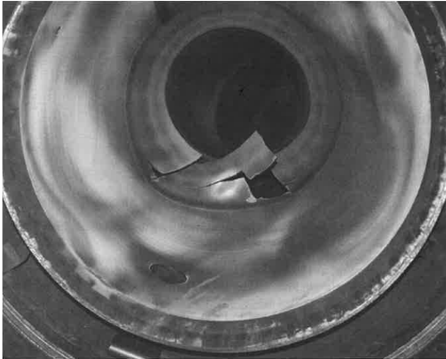
Figure 1.15: Combustion liner damaged by combustion instability [8].
