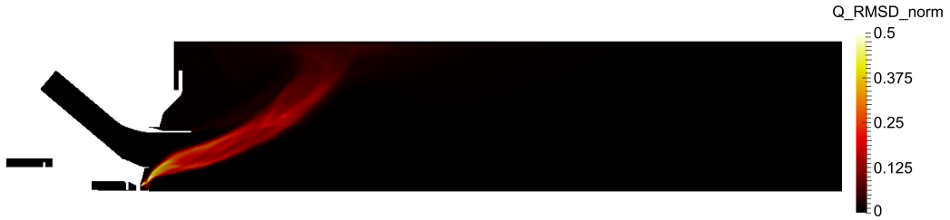
Figure 4.21: Normalised root mean square deviation of heat release; URANS simulations 30% excitation at frequency 1.05 St .
