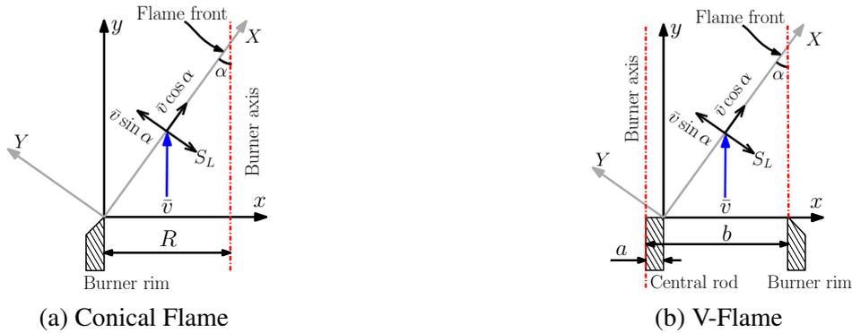
Figure 1: Schematic of different flame shapes
