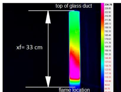
Fig 11: Thermal image of the glass tube with the V-flame inside it, for  $x_f = 33$  cm
