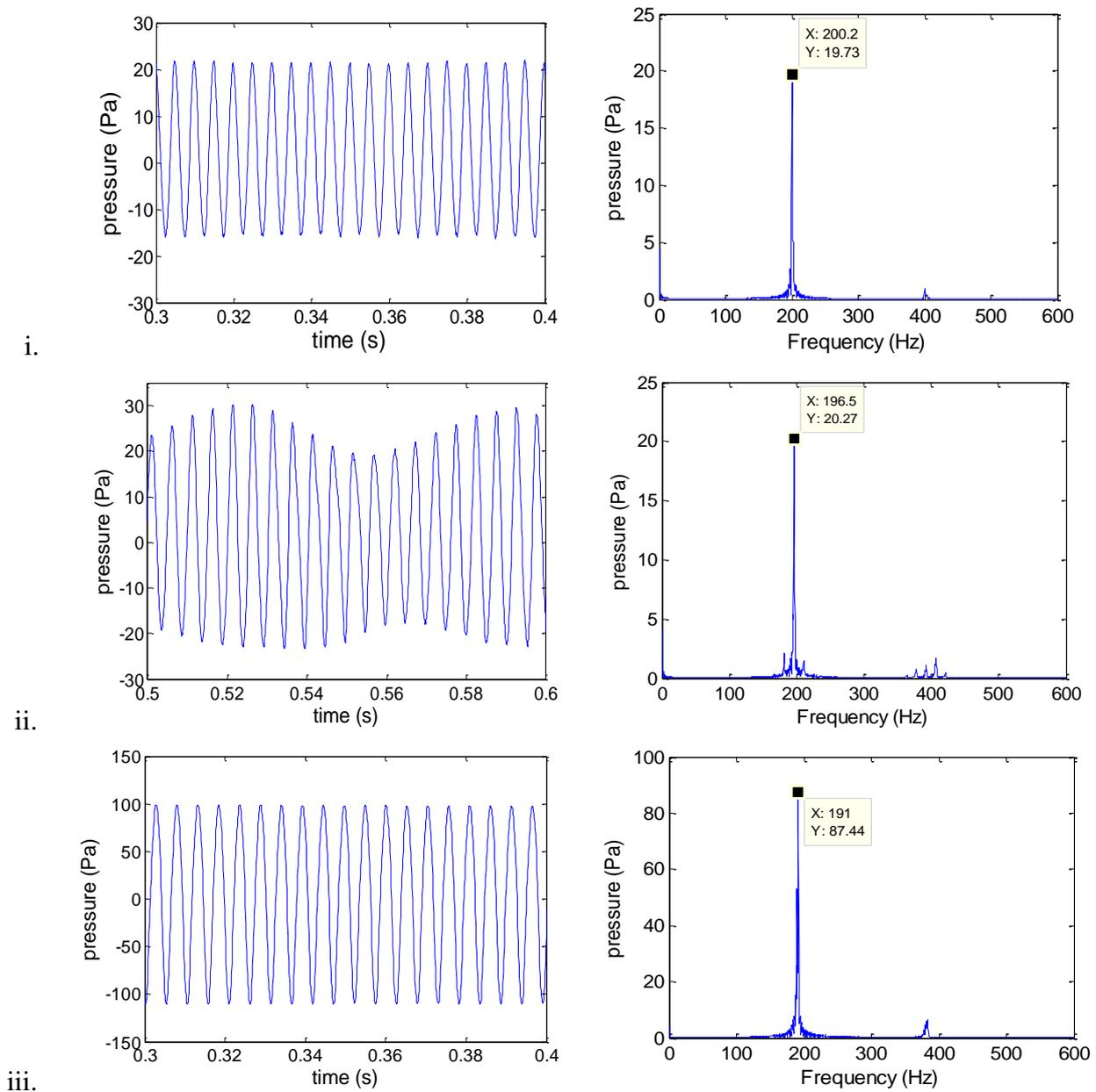
Fig 3: pressure-time series and FFT of the signal at (i)  $x_f=33$  cm, (ii)  $x_f=38$  cm and (iii)  $x_f=44$  cm
