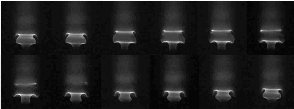
Fig 9: Flame oscillation pattern within a cycle for the high amplitude limit cycle
