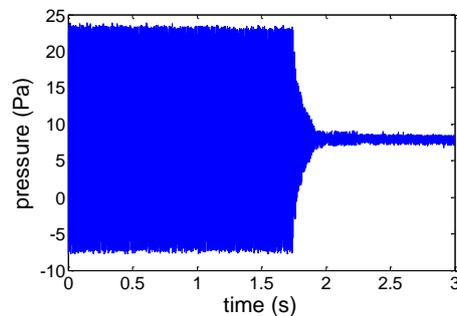
Fig 10: pressure-time history plot for damping measurement of the set-up
