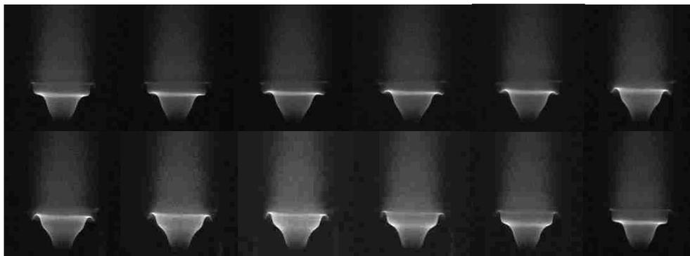
Fig 8: Flame oscillation pattern within a cycle for the transition phase
