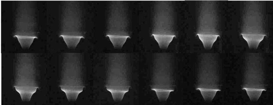
Fig 7: Flame oscillation pattern within a cycle for the low amplitude limit cycle
