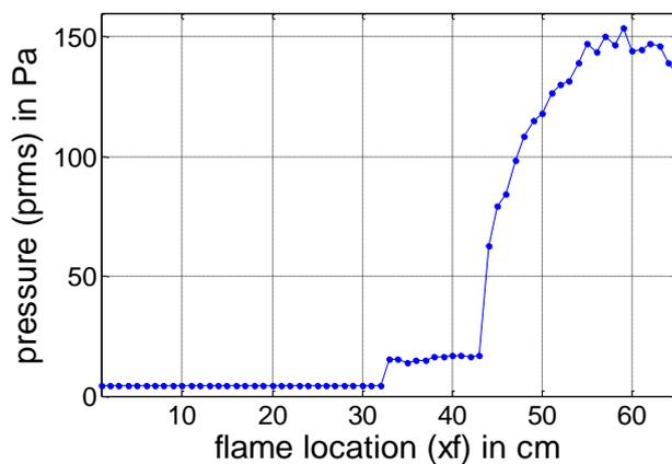
Fig 4: Bifurcation diagram (effect of flame location,  $x_f$  on r.m.s. pressure amplitude)
