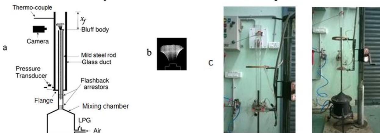
Fig 1: (a) Schematic of the experimental setup, (b) schematic of the V-flame and (c) the setup as installed in the laboratory (showing the glass tube with the traverse mechanism)
