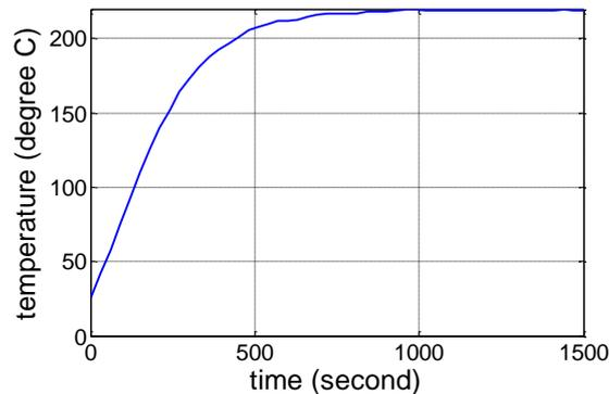
Fig 2: Temperature of the glass tube (measured at  $x_f=10$  cm) vs time
