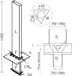
**Figure 1:** Burner geometry and close up of the bluff-body. Dimensions in mm. P: Plenum, F: Flame, L: Liner, B: Fuel injection holes, S: Pressure sensor, D: Damping orifices ( $\emptyset$ =4)
