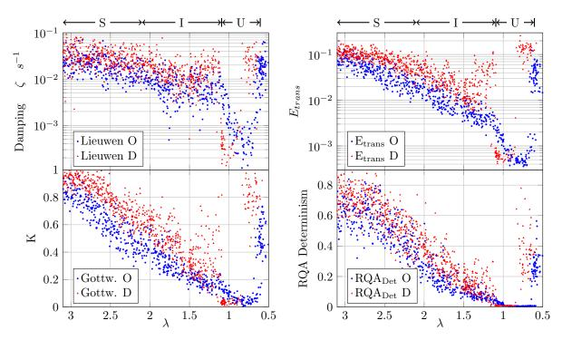
**Figure 4:** Stability margin results of both original (O) and damped (D) case, for the four investigated measures for slowly descending  $\lambda$ . Time windows of 0.8 seconds (4096 data points). Thermoacoustic state abbreviated to S(table), I(ntermittent) and U(nstable)
