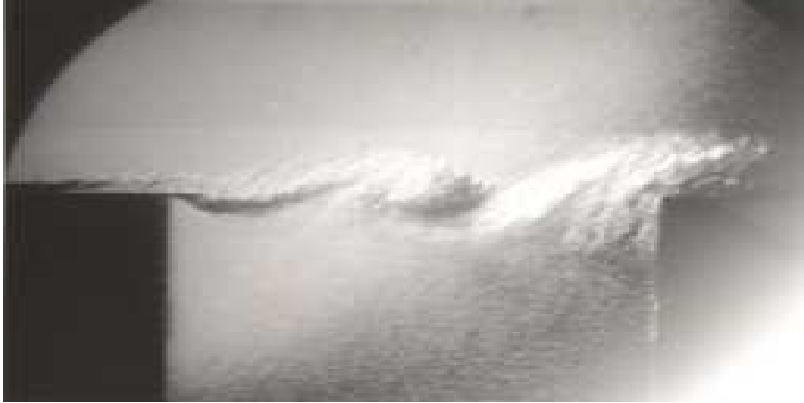
Figure 44: Visualization of vortical structures formed by acoustic perturbation of a shear layer at moderate amplitudes (second hydrodynamic mode).
