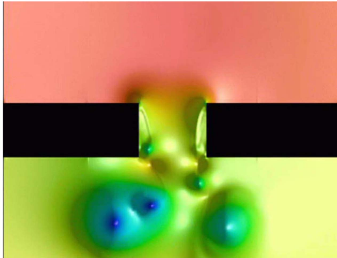
Fig. 28. Vortex shedding at a 90° slit.
