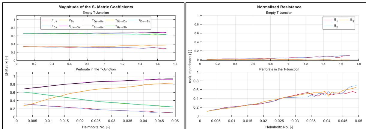
Figure 2 Characteristics of Empty T-junction and the perforate in absence of grazing flow; **a)** Magnitude of the S-Matrix coefficients, **b)** Normalised Resistance
