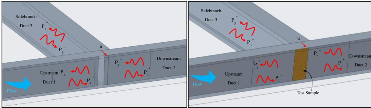
Figure 1 Schematic of the three-port experimental setup [6]; **a)** Empty T-Junction, **b)** Perforate at the intersection of the T-Junction
