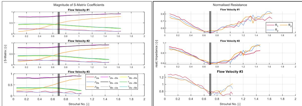
Figure 4 Perforated T-Junction acoustic characteristics at different flow speeds a) Magnitude of the S-Matrix coefficients, b) Normalised Resistance
