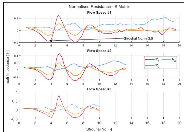
Figure 3 Normalised Resistance of empty T-Junction at different flow speeds
