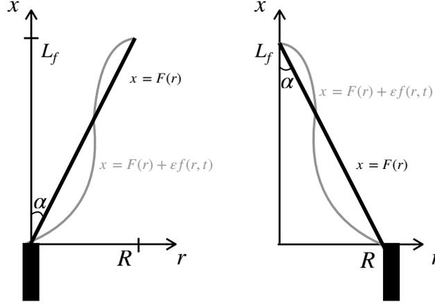
Figure 1: Sketch of the flames in the axisymmetric ref.system, (left) V-flame, (right) conical flame
