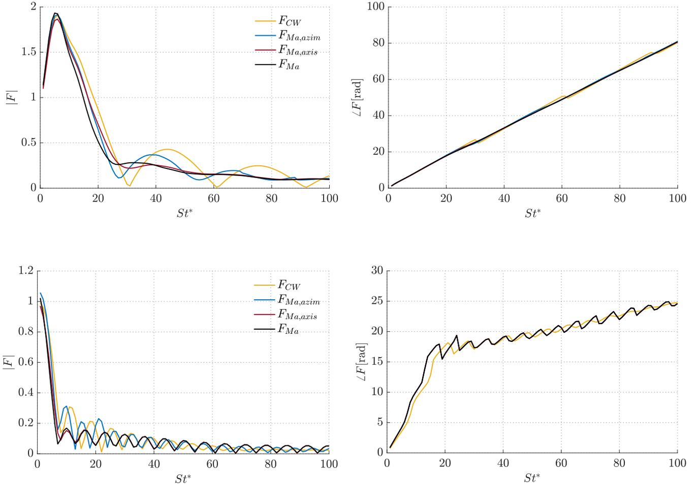
Figure 2: Gain (left) and Phases (right) considering no stretch ( $F_{CW}$  [3]), total stretch ( $F_{Ma}$ ) Eq.(3), axial only ( $F_{Ma,axis}$ ), azimuthal only ( $F_{Ma,azim}$ ). From top to bottom, angles are  $20^\circ$  and  $70^\circ$
