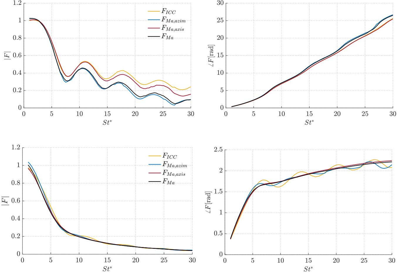
Figure 3: Gain (left) and phases (right) considering no stretch ( $F_{ICC}$  [8]), total stretch ( $F_{Ma}$ ) Eq.(3), axial only ( $F_{Ma,axis}$ ), azimuthal only ( $F_{Ma,azim}$ ). From top to bottom, angles are  $15^\circ$  and  $70^\circ$
