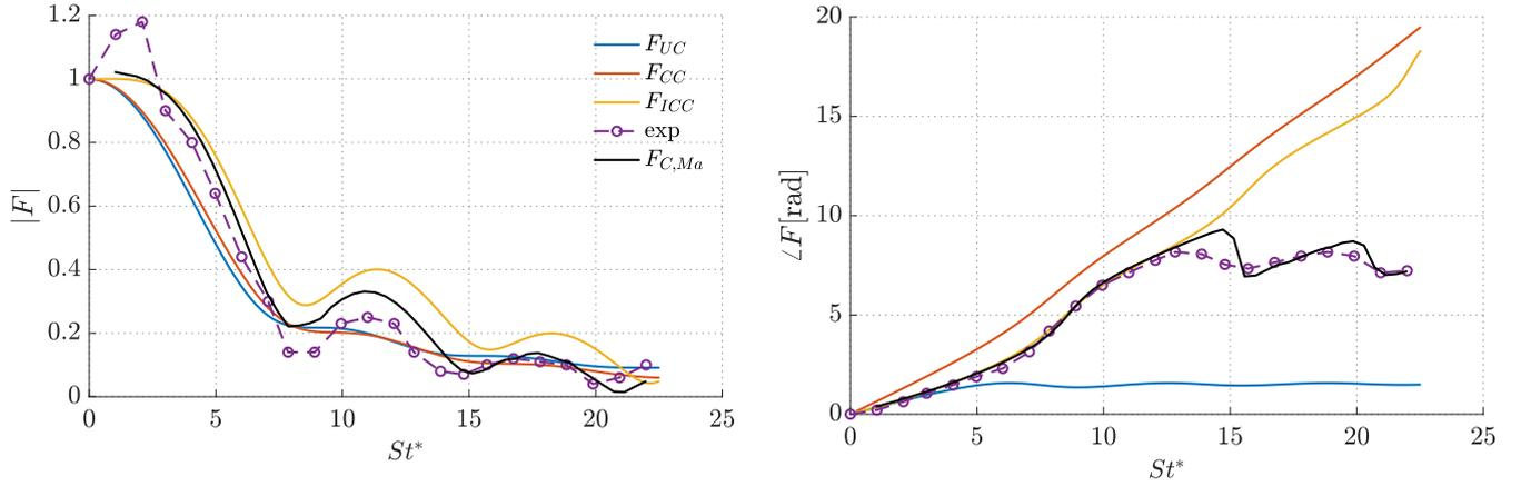
Figure 4: Gain (left) and Phases (right) considering FTFs with different velocity perturbation models:  $F_{UC}$  (uniform) Ducruix et al. [16],  $F_{CC}$  (convective) Schuller et al. [3],  $F_{ICC}$  (incompressible-convective) Cuquel et al. [8] with  $K = 0.8$ ,  $F_{C,Ma}$  (incompressible-convective) & azimuthal stretch from the present work.
