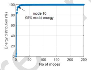
FIGURE 6: Cumulative energy distribution plotted for the combustor data for all possible model orders.
