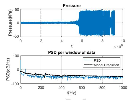
FIGURE 7: Combustor under normal operating conditions. Top: time domain combustor data; black line represents the position of the pressure-time trace, Bottom: Corresponding frequency spectrum for the window of time domain data; blue line represents FFT of the data and black line represents the spectrum from O<sup>3</sup>KID/ERA
